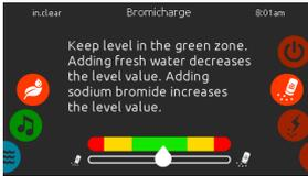
When performing a test, the BromiCharge™ gauge indicates the approximate sodium bromide level of the spa water.
