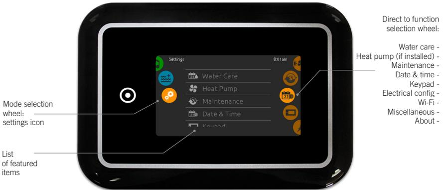
To select the settings mode, slide the left wheel up or down until the settings icon menu is highlighted in the middle.
