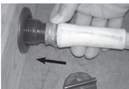
5. To disconnect the hose, push it in about one-half inch (1.27 cm) to shut off the water flow. Unscrew the hose.
